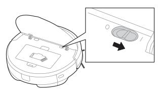
Step 5 Fill with the water and attach mop cloth to start mopping function.
